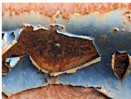
Scratches of coated surfaces often speed up corrosion – but not if the steel is coated with SmartCorr.
