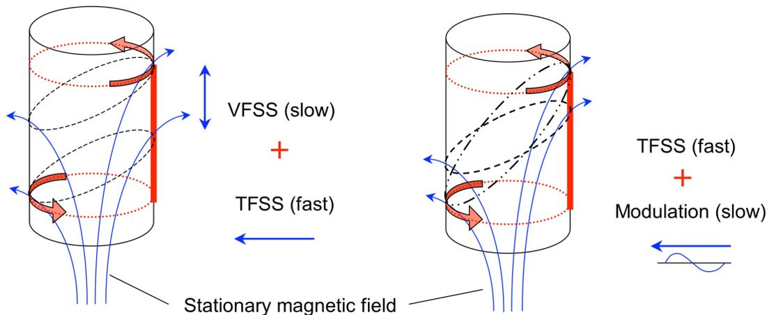
*Fig.3: Principle sketch (snapshot) of a TFSS with vertical magnetic field modulation (left, method (a)) and with amplitude modulation (right, method (b)). The dotted rings mark the upper and lower turning points of the fast rotating tilted ellipses. The rotation is indicated by arrows.*
