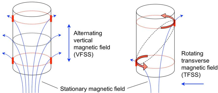
*Fig.1: Principle sketch of a Vertical magnetic Field Sweep System (left). The dotted rings mark the upper and lower turning points with collector sweeping, the central ring is the intersection area where the electrons hit the collector without sweeping. The Transverse Field Sweep System is sketched on the right. The intersection area is an ellipse, which rotates with the sweep frequency.*
