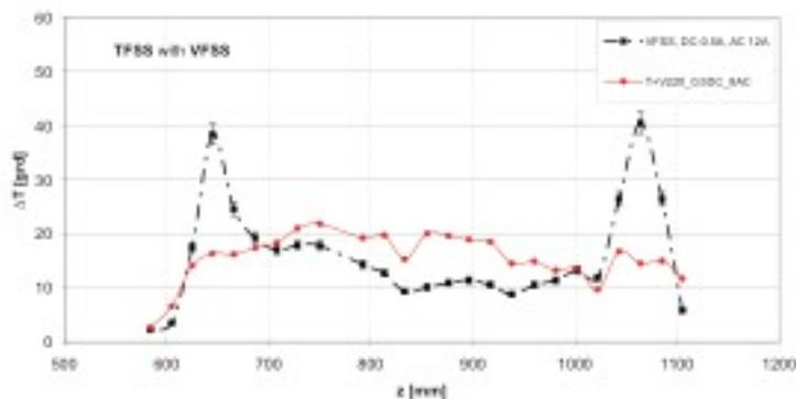
*Fig.5: Profiles of the collector temperature increase  $\Delta T$  along the vertical coordinate  $z$  for advanced sweeping: TFSS 3.5 A, VFSS 8 A, plus 0.5 A DC-current (dots). The profile for VFSS only is also shown for reference (squares).*
