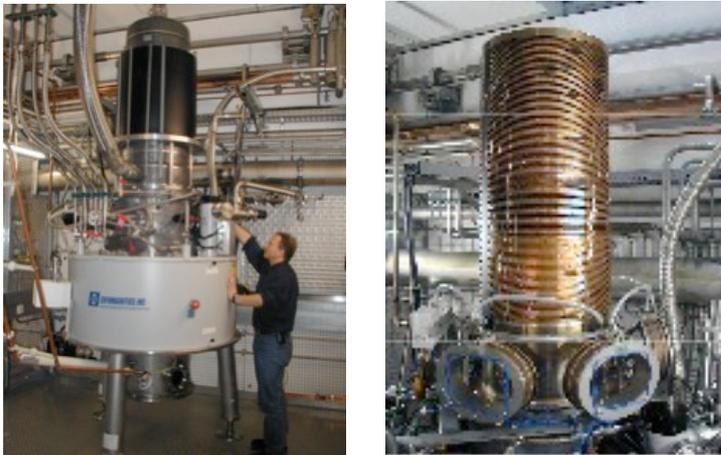
*Fig. 4. Left: The THALES Gyrotron. The normal conducting VF-coil (black) surrounding the collector is seen at the top part of the gyrotron.*
