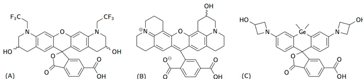
**Scheme 1:** Examples of the hydroxylated cell-permeating fluorescent dyes with a reactive carboxylic acid group for coupling to site specific ligands. Absorption/emission maxima (aqueous PBS buffer) are 532/553 nm (A), 574/597 nm (B) and 631/651 nm (C), respectively. Extinction coefficients are in the range of 60 000–80 000 m<sup>2</sup>/mol.
