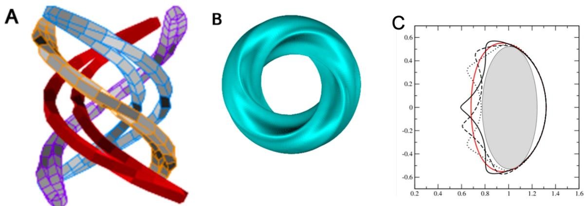
**Figure 1:** Hybrid Stellarator-Tokamak Design and Magnetic Field Configurations. **(A)** Four identical quasi-axisymmetric (QA) coils control the 3D shape of the magnetic field while maintaining a compact design. **(B)** The shape of the plasma boundary confined by the magnetic field configuration. **(C)** Poloidal cross sections of the plasma boundary produced by the magnetic field configuration.
