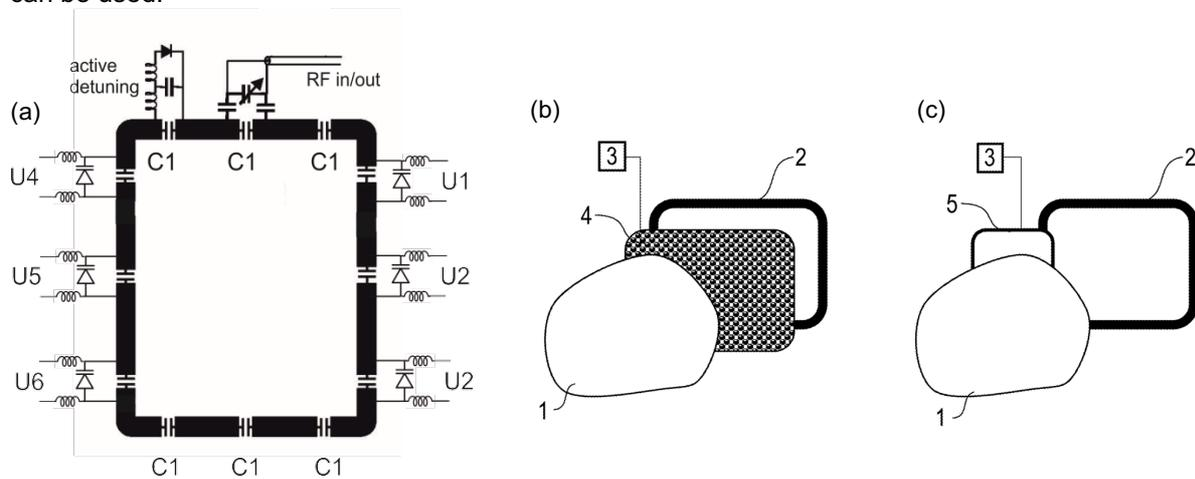
Fig. 2: Different implementations of the invention involving a sensitivity profile variation over time can be considered. The capacities in the RF coil can be varied quickly and independently when varactor diodes are used (a). Alternatively, metamaterials (b) or an auxiliary modulation coil (c) can be inserted between the sample and the RF coil to vary the sensitivity profile.
