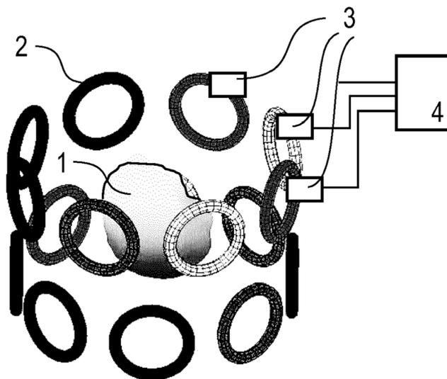
Fig. 1: As in common parallel MR imaging, the sample (1) is placed inside an arrangement of multiple RF receive coils (2) to detect the MR signal with additional spatial information. According to the invention each coil can additionally be equipped with an individual modulation device (3) to dynamically change the coils sensitivity profile. These profiles can be adjusted and monitored by a central modulation control unit (4).
