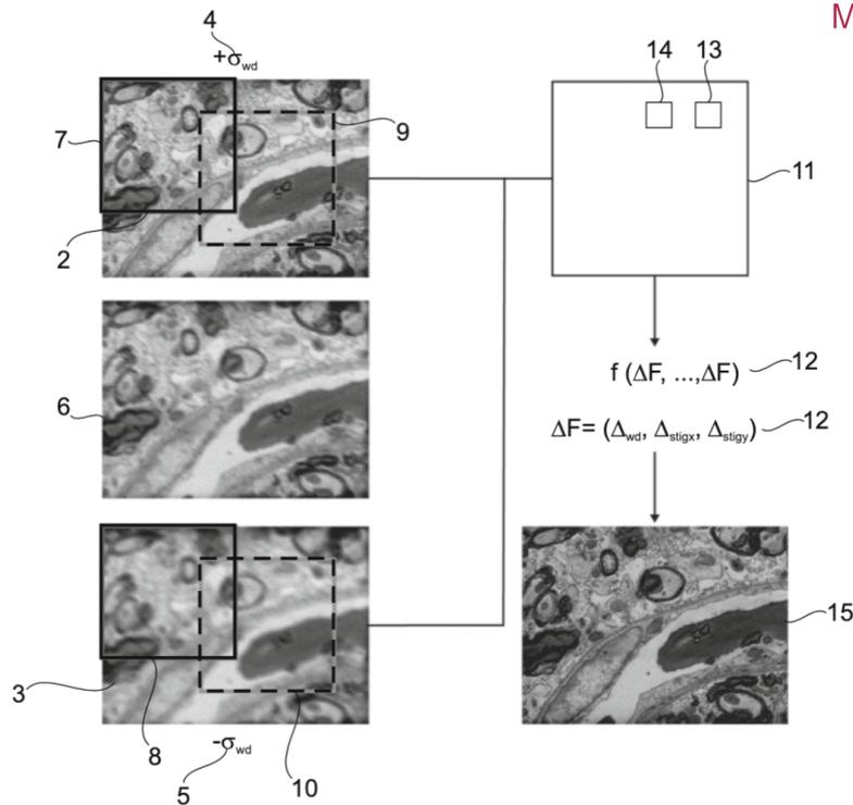
**Figure 2:** Workflow of the AI-based autofocus method: Two perturbed images (2, 3) with known deviations in working distance are compared to the flawed image (6). Corresponding patches (7/8 and 9/10) are analyzed by the processing unit (11), which predicts corrections (12) for focus and astigmatism. The optimized settings result in an improved image (15).
