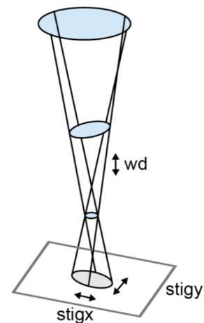
**Figure 1:** Visualization of key electron microscopy parameters: working distance (wd) controls focus depth, while stigx and stigy correct horizontal and vertical astigmatism to improve image sharpness.
