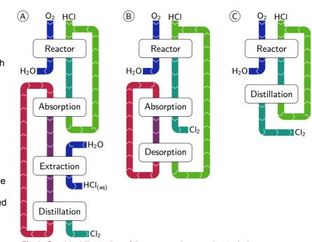
**Fig 1:** Graphical illustration of the proposed separation techniques: **A**: Absorption & Extraction, red: organic solvent cycle; **B**: Absorption with Ionic Liquid (red); **C**: Direct Distillation.
