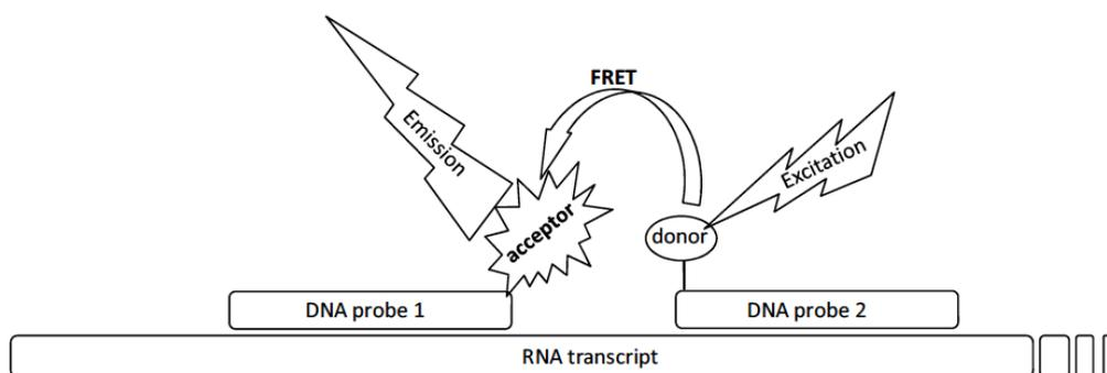
Figure 1: Schematic overview of the invented method of detection of nucleotide polymerase activity, consisting of specific, functionalized DNA-probes to serve as fluorescence donors and acceptors in a time-resolved fluorescence energy transfer (FRET) assay.
