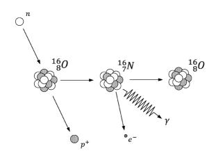
Fig. 1: <sup>16</sup>N nuclei in the cooling water can absorb the fission neutrons inside the reactor core releasing a proton. The formed <sup>16</sup>N nucleus decays and emits a gamma particle that can reach the detector
