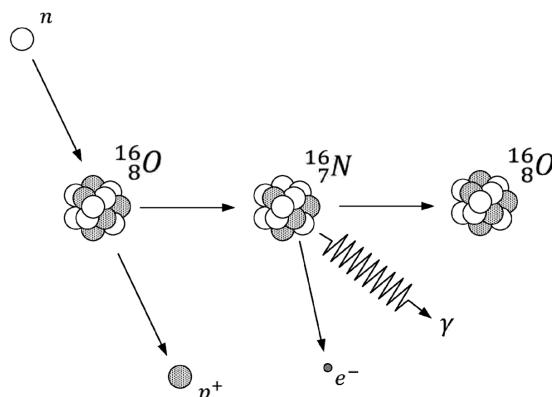
Fig. 1:  $^{16}\text{N}$  nuclei in the cooling water can absorb the fission neutrons inside the reactor core releasing a proton. The formed  $^{16}\text{N}$  nucleus decays and emits a gamma particle that can reach the detector
