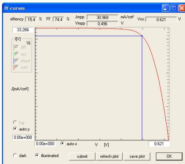
Fig. 2: Screenshot showing the simulated *I-V* curve for a position or region selected in the main window as calculated by *Local I-V 2*.
