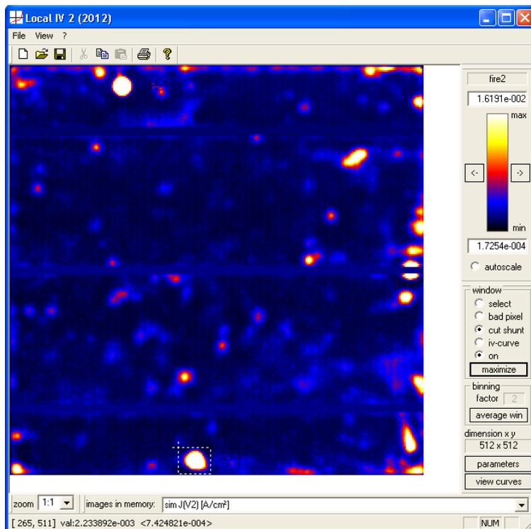
Fig. 1: Screenshot of the main window of *Local I-V 2* with a simulated current density image displayed.
