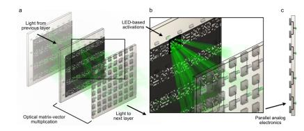
onto a 2D array of photodiodes. (PDs) (c) An electronic board contains a parallel array of neurons each associated with a pair of PDs representing the positive and negative inputs to the neuron.
