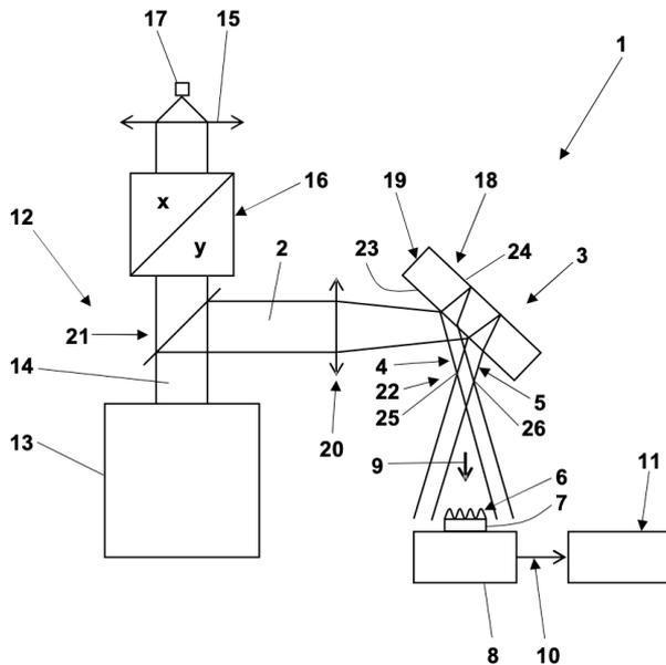
Fig. 3: Example of an implementation, according to the invention, of a shear-interferometer into a laser-scanning microscope.
