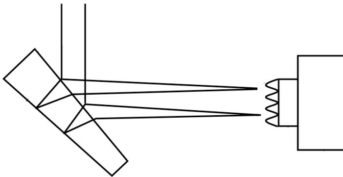
Fig.1: Simplified beam paths of a possible implementation of the invention using a Shear-Interferometer
