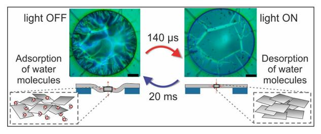
Fig. 1: Scheme incl. optical images of photo-actuation for free-standing PDA film (black scale bar is 10µm). [1]
