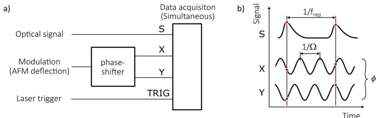
**Fig. 1:** Brief overview of the signal processing method. **a)** Besides the optical signal from the microscope tip  $S$  and a laser trigger ( $TRIG$ ), the modulation signal is copied and phase shifted to form the pair  $(X, Y)$ . **b)** The signals  $X$  and  $Y$  are sampled at the laser repetition rate entered by a trigger. From  $X$  and  $Y$  a phase relation can be obtained instantaneously for every sample.
