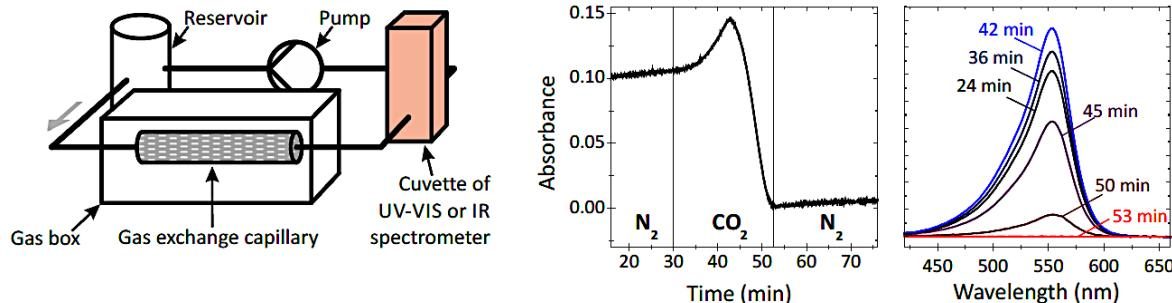
A very efficient gas exchange through the superamphiphobic membrane could be shown.
