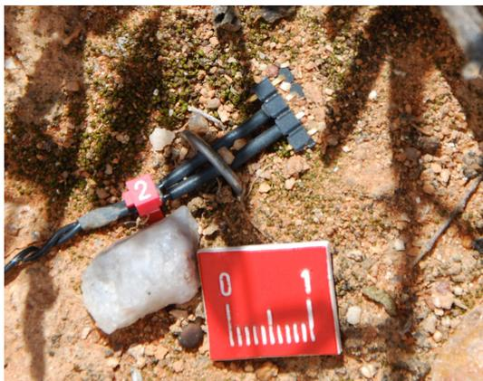
**Fig. 1:** Example of one water content sensor within soil.
